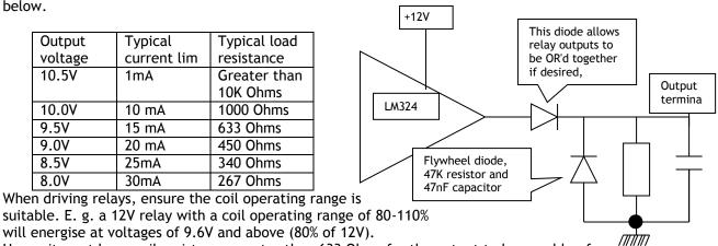
Hence it must have coil resistance greater than 633 Ohms for the output to be capable of achieving the desired voltage. A suitable UL approved relay is Hongfa type HF41F/9.
