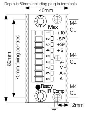
Remove plug on terminals, and plastic cover to gain access to the fixing holes
