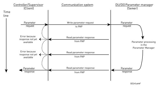
Figure 8. Data flow for Base Mode Parameter Access
