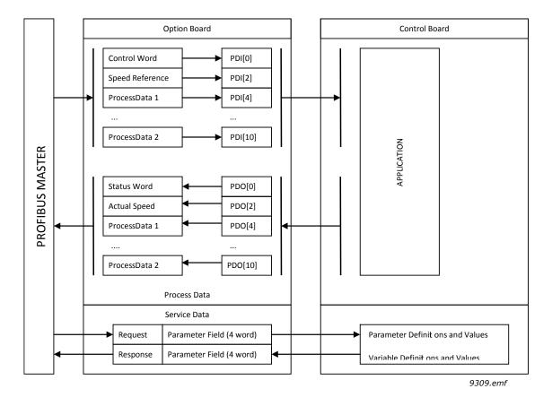
Figure 6. Data transfer between PROFIBUS master and Vacon 100
