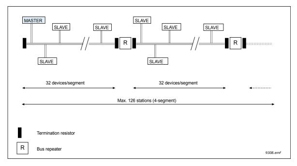
Figure 1.Cabling and bus termination
