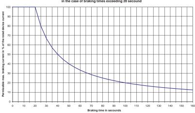
Reduction of the permissible max. braking current in the case of braking times exceeding 20 secound
