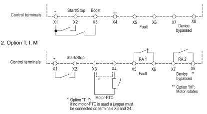
The input resistance of the control inputs is ca. 10kOhm. To control them, it is necessary to use switching contacts enabling reliable switching of the lower control currents (e.g., AgNi+Au)!
