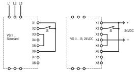
Afterwards, the supply voltage is to be switched on. No motor must be connected! In the case of standard devices via L1, L2 and L3; and in devices with option "B" via 24VDC or 230VAC. After a short period of time, the yellow LED flashes with a different frequency, depending on the reset mode adjusted.
