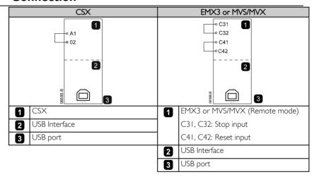
CSX: For the USB Interface to accept serial commands, a link must be fitted across terminals A1-02 on the soft starter.
